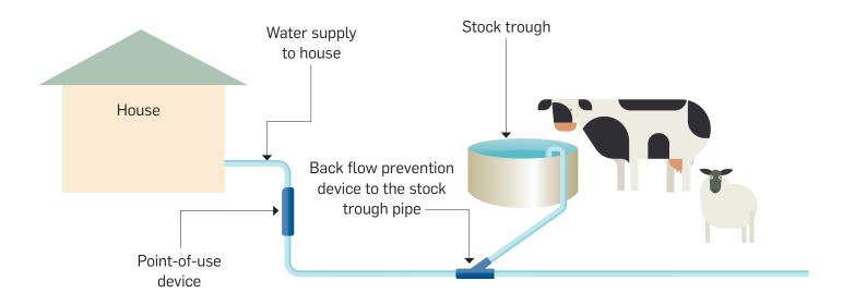
An alternative is to treat water for drinking and cooking purposes only. For this, a bench-top or under- sink pointof-use device can be used, or water can be boiled. However, it must be made clear that water from the other taps is unsuitable for drinking.
