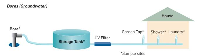
The intake (bore) is an important part of your system. Usually, providing a good intake is only a little more expensive than a poor one, yet a good intake will fix many of the problems caused by turbidity and other contaminants.
