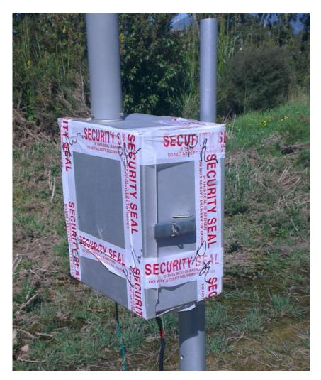
Photo 1 Photograph of the monitoring station at site Z-4 illustrating the security tape on the device with signatures of the field technicians across all joins. The sample filter is situated inside the metal case.
