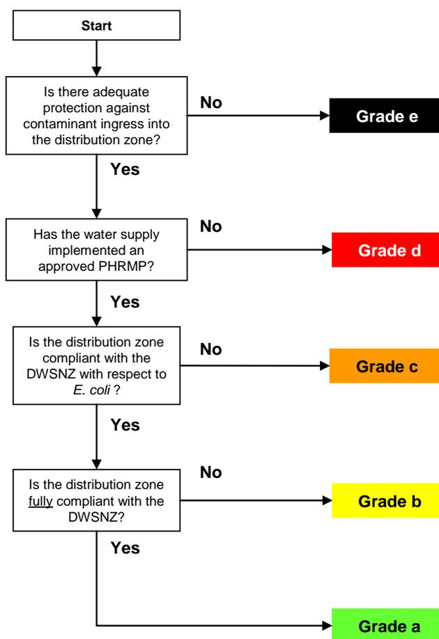
**Fig. 5.2 Derivation of distribution zone grades – Model 3**
