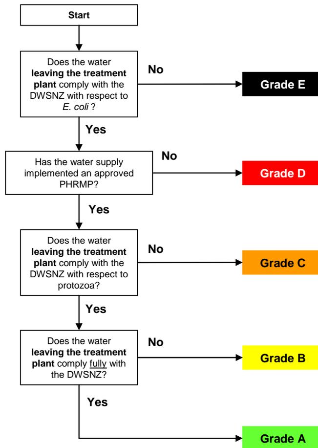
**Fig. 5.1 Derivation of source-treatment plant grades – Model 3**
