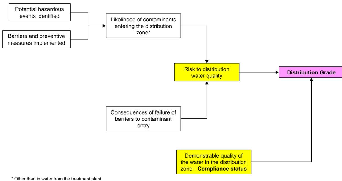
Fig. 3.2 Overview of the distribution zone grading framework - Model 1
