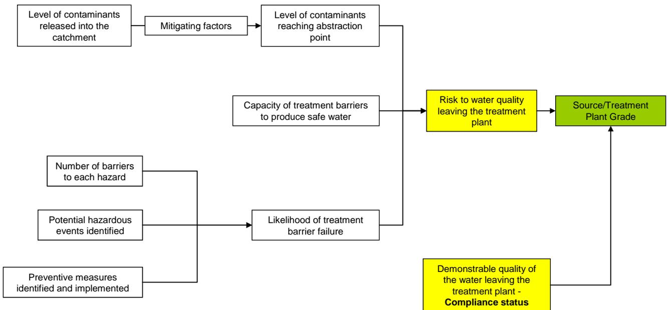
**Fig. 3.1 Conceptual basis for the source-treatment plant grading - Model 1**
